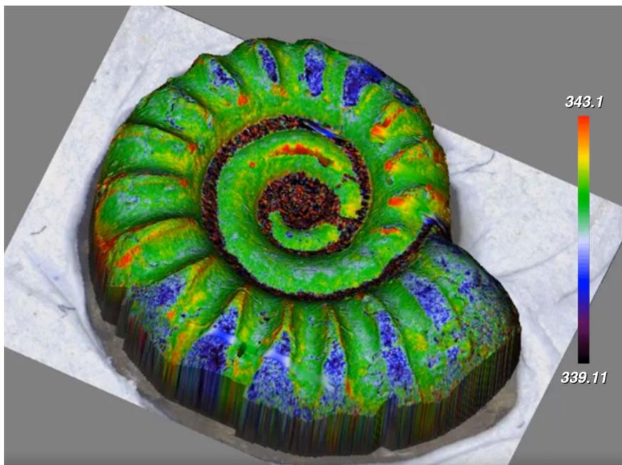
StreamLine imaging and LiveTrack focus-tracking technologies were used to produce a topographic Raman image of an ammonite fossil. This sample is large and has an extremely complex surface topography, making measurement impossible for most other Raman systems. Variations in Raman band positions from iron sulfide indicate regions of higher compressive stress (red) and higher tensile stress (blue).
