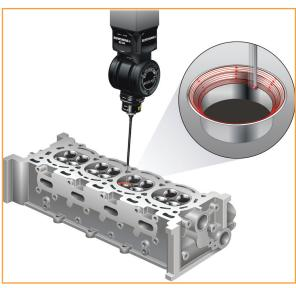
REVO® valve seat and stem scanning on generic head
