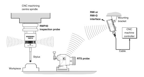
Radio transmission does not require line-of-sight between the probe and transmitter, and will pass through very small gaps and machine tool windows. This allows easy installation, either inside or outside the machine enclosure.
