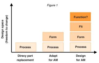
How many of these AM capabilities we can exploit, and how much benefit we can accrue, will depend on the level of freedom or constraint that we are operating under. Another way of thinking about this is the size of the 'design space' within which we can optimise our design (see Figure 1).
