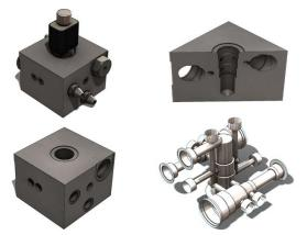
The benefits of this simple approach are that the design phase is relatively straightforward and that the manufacturing cycle time for this simple circuit is short. The limitations are that we get sub-optimal fluid transfer performance due to the cross-drilled pipe network, the part is massive and therefore compromises product performance whilst using material inefficiently, and that we require eight additional pressure plug parts to complete the assembly.
