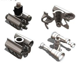
So good progress. However, there are still some limitations. Horizontal passages need supports, and we must leave sufficient material on for finish machining. We also find that such lightweight parts are naturally less rigid than their more massive counterparts, and this can complicate the finish machining process.
