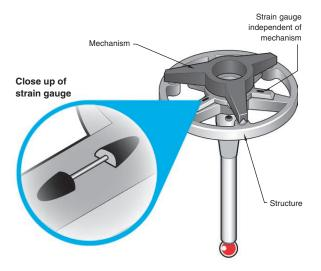
Sensing is independent of the probe mechanism which means that probes with Rengage technology provide capabilities not associated with conventional design.
