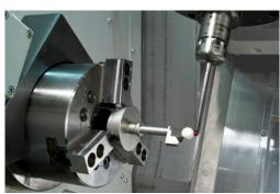
AxiSet Check-up V2 with support for checking rotary axis alignments of mill-turn machine tools
