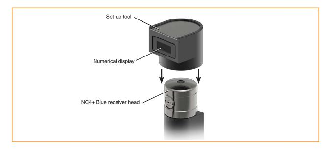
NOTE: Excessive cutting fluid deposits on the NC4+ Blue receiver may prevent the set-up tool from switching on. It may be necessary to clean the top of the NC4+ Blue receiver to ensure good electrical contact to the set-up tool.
