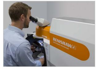
Renishaw inVia Qontor® confocal Raman microscope
