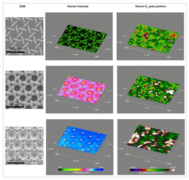
Figure 5. SEM and Raman images collected from the sample, z=0  $\mu$ m is the surface. Raman intensity images illustrate the microstructure of the sample and correlate well with the SEM images. The peak position of the E2 band moves towards the stress-free value at the surface. The Raman measurement area was 38.1  $\mu$ m  $\times$  26.1  $\mu$ m  $\times$  14  $\mu$ m, with a step size 0.3  $\mu$ m  $\times$  2  $\mu$ m.
