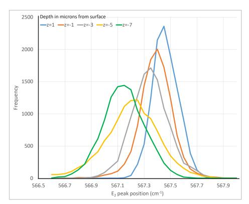
Figure 6. Histogram illustrating the variation in  $E_2$  peak position for different depths in the structure. The typical peak position upshifts towards the stress-free value, 567.5 cm $^{-1}$  and the distribution sharpens when moving from bulk to the surface of the sample.
