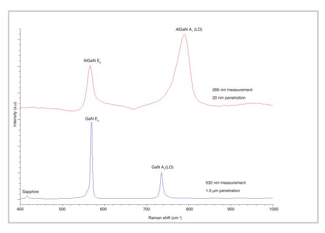
Figure 1. Raman spectra of different layers in a AlGaN/GaN heterostructure. The depth probed by Raman spectroscopy is dependent on the excitation wavelength. Here a UV excitation laser is used allowing the ultrathin AlGaN layer to be measured.
