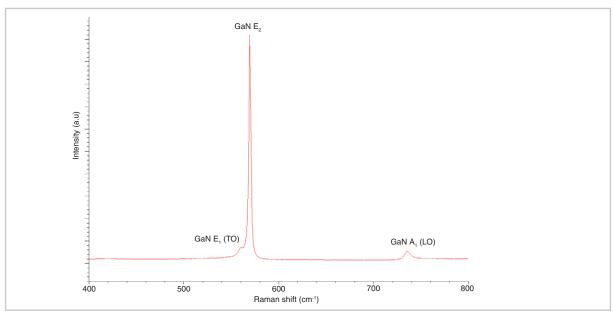
Figure 4. A typical spectrum from the novel nanostructure with GaN Raman modes labelled. The E,(TO) mode is present due to off axis growth of the material.
