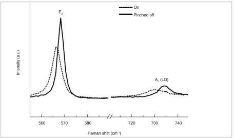
Figure 7. Comparison of Raman spectra for an on (hot) and pinched off device (cold).
