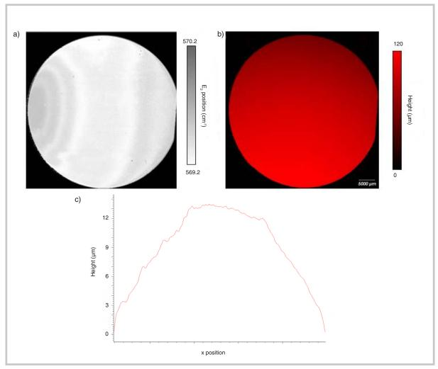
Figure 3. a) peak position of the  $E_2$  mode illustrating stress across the wafer, b) topography image collected during Raman measurement, c) wafer bow (wafer tilt subtracted).
