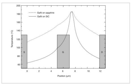
Figure 8. Temperature distribution of HEMTs fabricated on sapphire and SiC substrates. Devices were operated at different power densities to produce a peak temperature of 180 °C.
